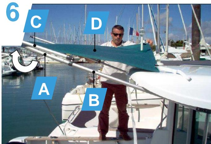
Once you have attached the awning to the lower part of the wheelhouse, fold the remaining part onto the roof to attach it. If your wheelhouse has a VHF antenna, you will see that a notch has been provided to allow it to pass through the canvas.
